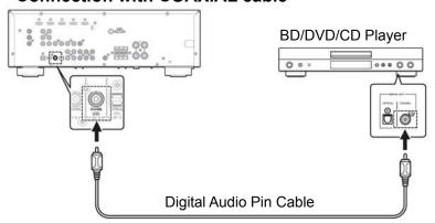
Picture shows an example of the connection. Depending on your BD/DVD/CD player's digital output, connect the receiver with either optical or coaxial.
