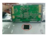
3. There is a marker on the place where the black cushion was. At the bottom of this marker, pile two pieces of "Himeron" tape to a total height of 1 mm.
